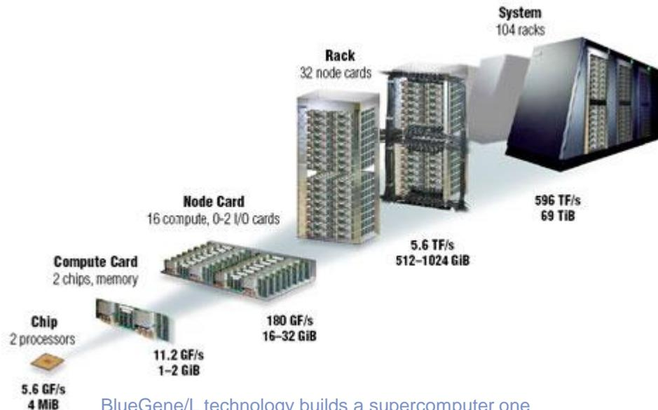
BlueGene/L technology builds a supercomputer one dual-processor chip at a time. Chips are aggregated into compute cards, which are then assembled into node cards. Each rack holds 2 node cards, and the full machine now comprises 104 racks.
